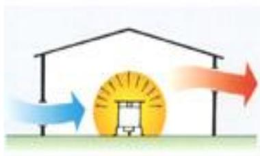
Gases are heavier than air and closed tentage in the case of gas leaks would entrap a layer of gas at low level. (See section on Carbon Monoxide poisoning).
