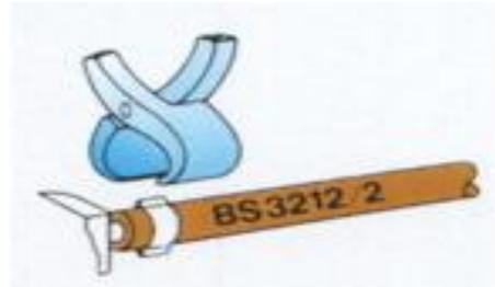
Make sure that the hoses are kept clear of 'hot spots' and inspect them from time to time. Replace any hose that shows signs of wear, cracking, corrosion, rusting or other damage. Keep hose lengths as short as possible for your particular set up.
