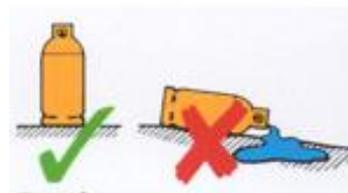
Cylinders should be placed upright and outside the confines of the cooking tentage so the cylinder valve is more accessible in the event of a fire. Allow enough hose for this. Bottles should not be kept under a cooking table as, should a fire start, you cannot get to the bottle to turn off the supply without going under the fire itself.
