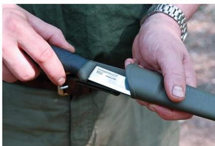
This image shows poor technique. There is every chance that the fingers of the holding hand would be cut by the knife as it is withdrawn from the sheath.
